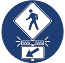
Rectangular Rapid Flashing Beacons (RRFB)
