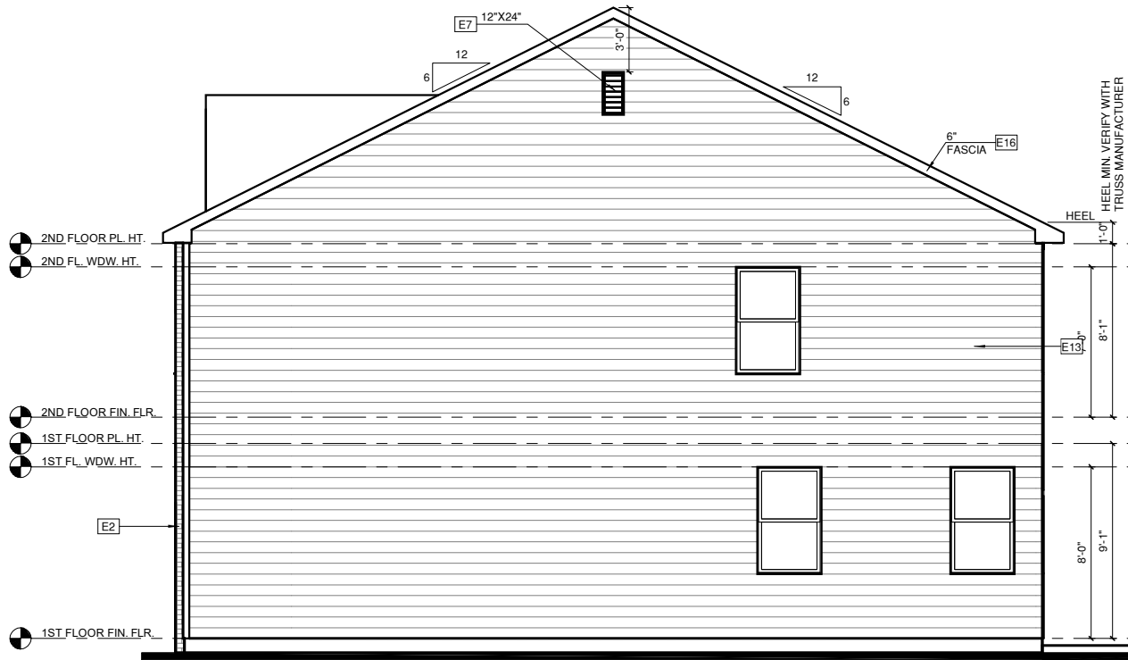
RIGHT ELEVATION 'I' AT END UNIT CONDITION
