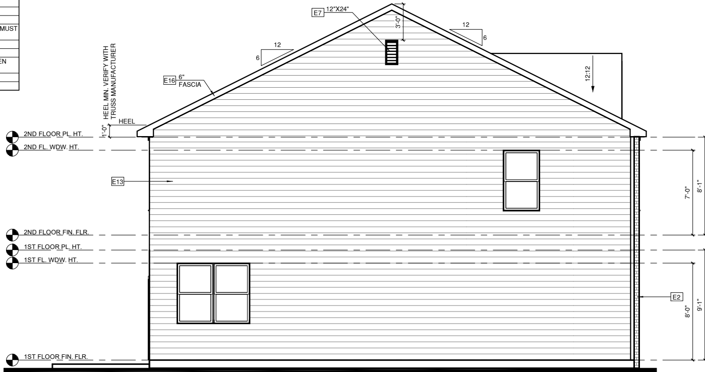
LEFT ELEVATION 'H' AT END UNIT CONDITION
