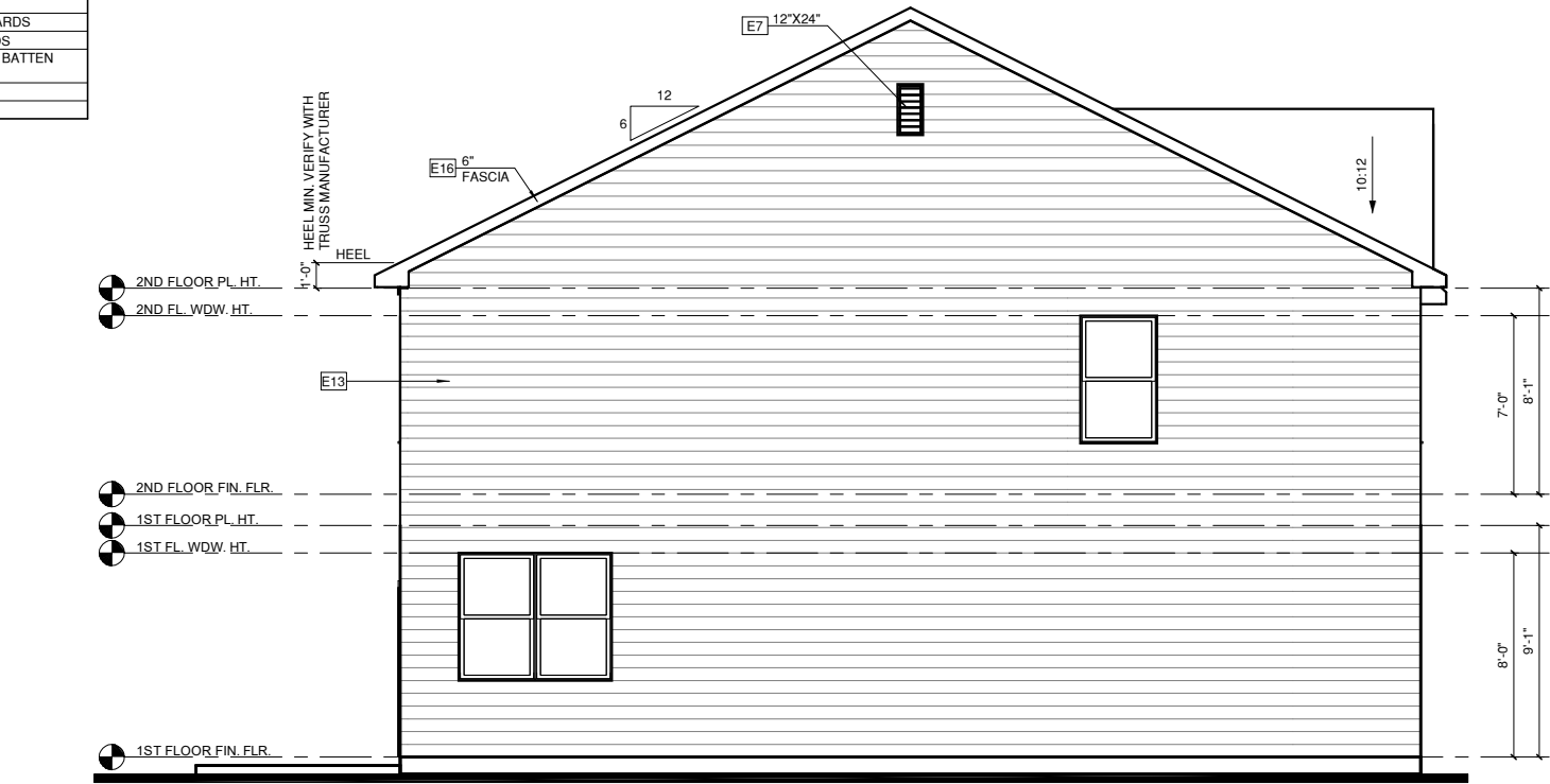
LEFT ELEVATION 'B' AT END UNIT CONDITION
