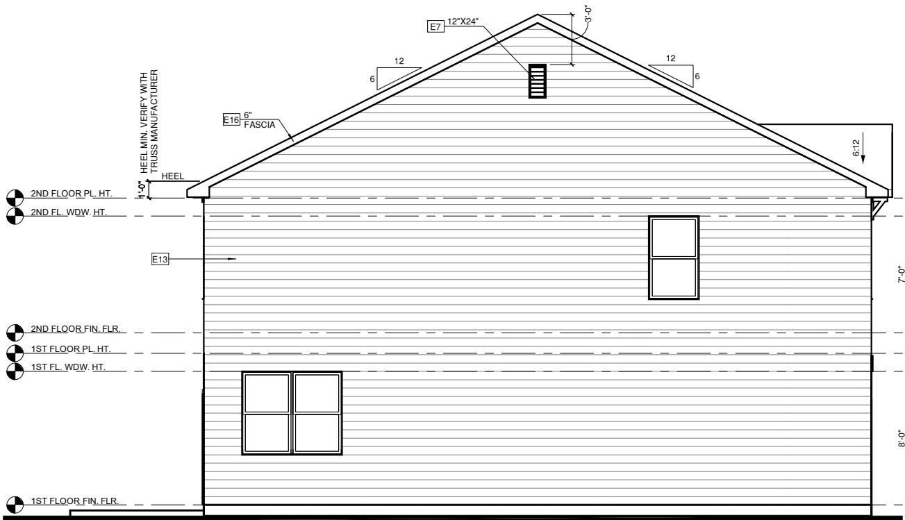
LEFT ELEVATION 'L' AT END UNIT CONDITION
