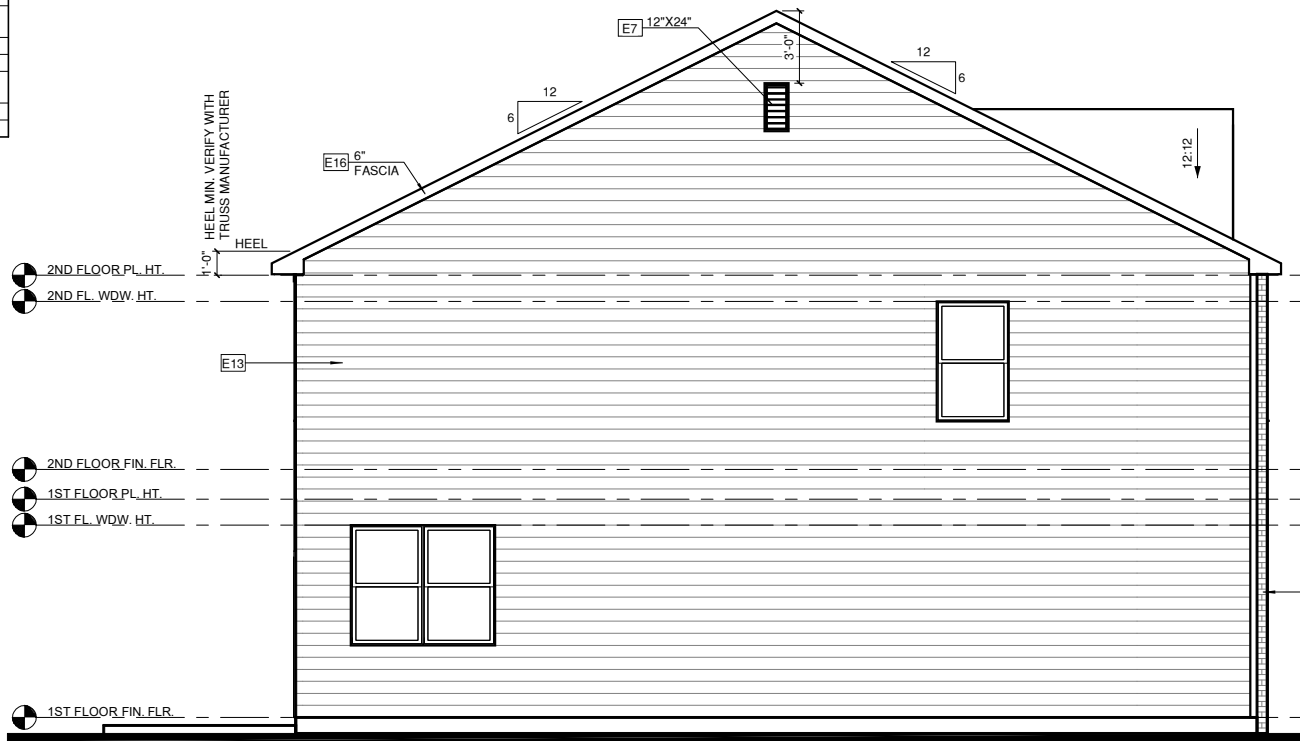
LEFT ELEVATION 'I' AT END UNIT CONDITION
